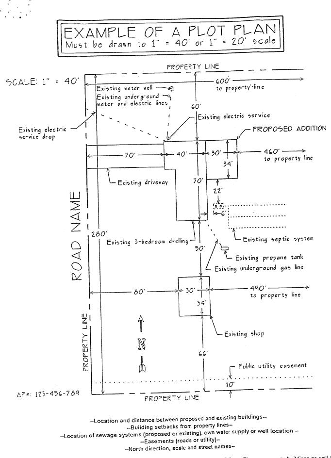
Make a complete plot plan even if you are only building an addition to an existing building. Show accessory buildings as well as the proposed addition, as this is important in determining your compliance with lot coverage regulations.
