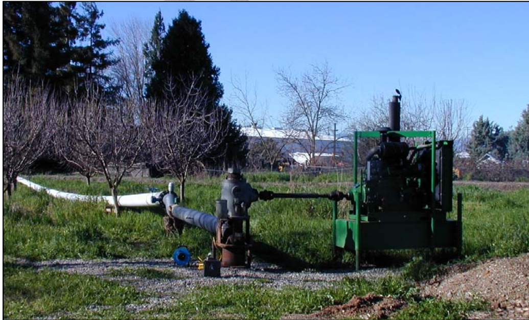
Photo 1. Test Production Well and Test Pump with Conveyance Pipe.
