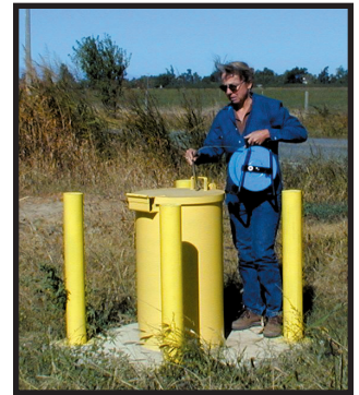
Figure 4. Using an electric well sounding device to measure the depth of groundwater at a triple completion, dedicated observation well.
