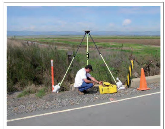
Figure 5. Benchmark or "geodetic" station used to re-level ground surface elevations and monitor subsidence.
